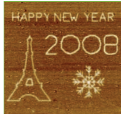
30µm scan of a lithography pattern created by charge deposition on Si sample. An Agilent AFM retrofitted with a 100x100µm nPoint scanner was used. Courtesy of ScienTec (France).
