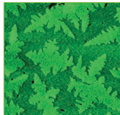
TappingMode™ image of pentacene dendrites on a silicon dioxide substrate acquired with a MultiMode® AFM. Scan size = 11 µm. Image courtesy of Frisbie Group, University of Minnesota.
